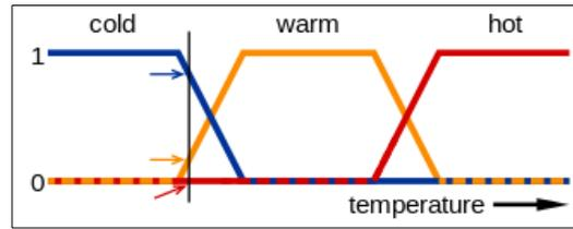
Figure 1: Illustration of Fuzzy Logic
